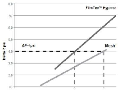
Pressure Drop versus Feed Flow for Mesh wrap and FilmTec™ Hypershell™ 8038 elements. FilmTec™ Hypershell™ has less exterior bypassing and requires approximately 30% less flow than mesh wrap for an equivalent pressure drop.
